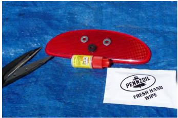
Clean the back of the reflector and the washers to remove the dust and any oil. I used a Penzoil Hand Wipe designed to take grease off skin.
